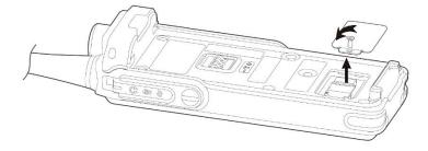
2. Install the TF card, put the card slot cover back in place, and then tighten the screw.
