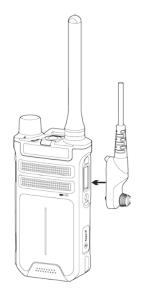
3. Tighten the screw on the audio accessory plug.
