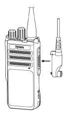
3. Tighten the screw on the audio accessory plug.
