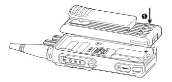
2. Press and push the battery into the battery slot until a click is heard.
