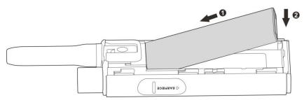
3. Place the hooks of battery cover to the slots, and then push the battery cover upwards until you hear a click.
